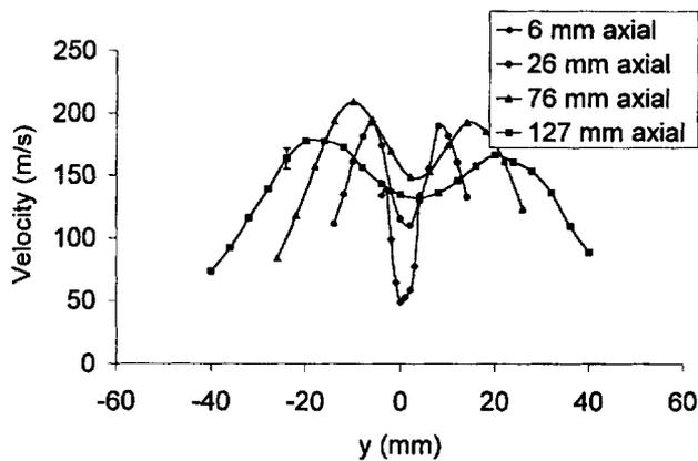
Fig. 7 Cross-sectional particle velocity profiles, 200 amp/60 psi
