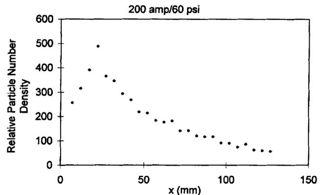
Fig. 2 Centerline particle number density, 200 amp/60 psi
