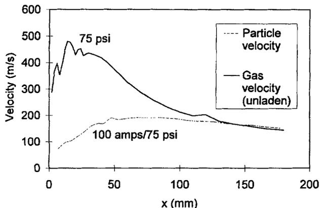
Fig. 8 Centerline air velocity for unladen flow, 75 psi
