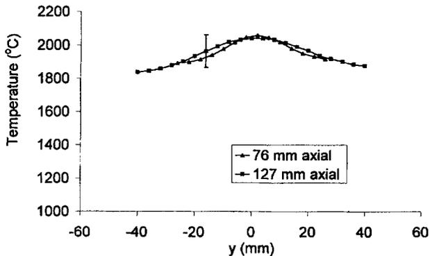
Fig. 11 Cross-sectional particle temperature profiles, 200 amp/60 psi
