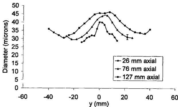
Fig. 5 Cross-sectional particle size profiles, 200 amp/60 psi
